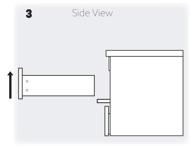
Once the screws are removed, gently lift the drawer up and out of the cabinet.
