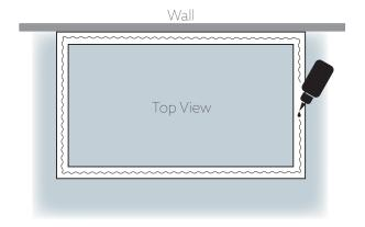
Using non-acidic silicone, apply a continuous bead of silicone to the top four edges of the vanity and at the back where the top meets the wall. Position the top so that it has equal overhang on each side, ensuring the top surface is level.
