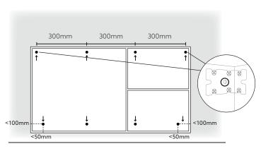
To securely fasten a vanity to the wall, use appropriate screws or bolts at the top and bottom of the cabinet. Use top left and right brackets and evenly space horizontal fixings no more than 300mm apart. For the bottom, start fixing points no more than 100mm from each end and no higher than 50mm from the base panel.
