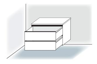
Install drawers and doors back onto the cabinet and make adjustments to align the doors and drawers correctly. Remember that it is the responsibility of the installer to make any adjustments to drawers and doors after installation. Don't forget to remove the transportation blocks on the underside of the cabinet.
