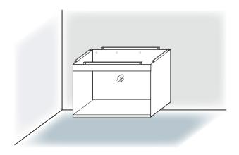
For wall hung vanities, position the vanity over the pipes in the correct position and fix it with a single screw in the center of the vanity to hold it in place. Make sure that the vanity is completely level. You may want to use a level support/noggin to assist while levelling.
