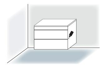
Apply non-acidic silicone to all edges where the vanity top and cabinet meet the wall and floor. Remember that materials used in the construction of this unit are water-resistant, not waterproof, so all areas need to be sealed to prevent water penetration. You can use gap sealant in place of silicone where the unit meets tiled surfaces.
