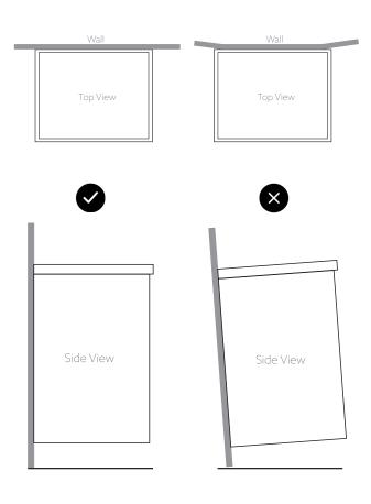
Before installation, ensure that both the wall and floor are plumb and level, respectively. Failure to do so may result in the following issues:
