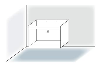
Remove all doors and drawers from the cabinet. Measure the correct plumbing locations and drill holes for plumbing in the back panel and/or base of the cabinet using an appropriate-sized hole saw.
