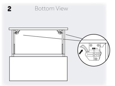
The lever is located at the bottom of the drawer.
