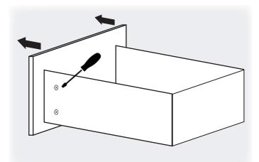
To remove drawer front penal, turn two screws on each side first and pull drawer front dorwards.
