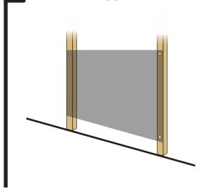
For wall hung vanity and basins, a support beam must be fixed between the studs to provide a solid wall backing.
