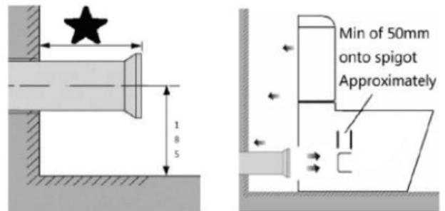
**Step 2: Do the below installation for the cistern fixing.**
