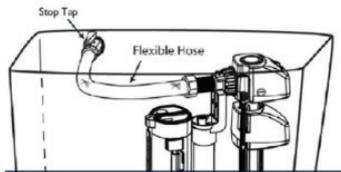
**Fit off stop tap then connect rear water inlet valve to stop tap. Fill cistern and ensure correct water level.**
