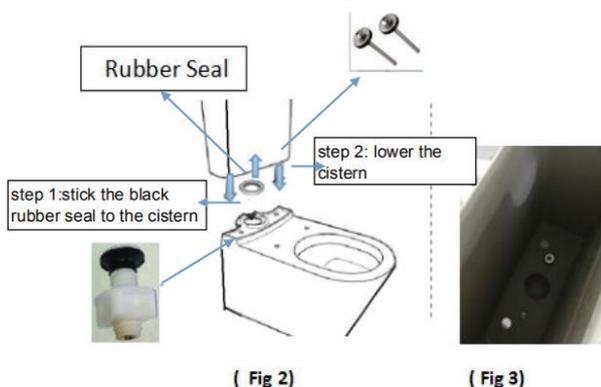
**\*Before fitting cistern to ensure all cistern seal nuts are tight.**
