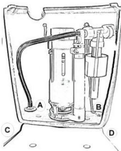
**Remove cap from cistern plug A or B at base cistern. Connect flexible hose to cistern plug A or B depending on location of stop tap. Complete stop tap connection to underside of cistern plug A or B. Fill cistern and ensure correct water level. Note: Inlet valve can be adjusted if required.**
